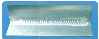
• As concentration of arc is excellent, welding is performed effectively for fillet (overlapping) joint welding for thin aluminum plates.
